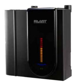
The FAAST XM aspirating smoke detector combines dual source (blue LED and infra-red laser) optical smoke detection with advanced algorithms to detect a wide range of fires while maintaining enhanced immunity to nuisance particulates. This enables FAAST XM to accurately detect incipient fire conditions as early as 30 to 60 minutes before a fire actually starts for Early Warning Fire Detection and Very Early Warning Fire Detection.
